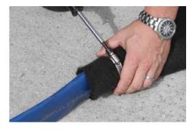
Step 5. Tighten the clamp so that it firmly secures the sock to the hose. The clamp should be tight enough so that no excess water or materials are flowing out of the sock during the filtration process.
