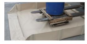
Install or place equipment into the containment area. If a spill occurs, foam wall ends should rise up as the area fills with liquid.
