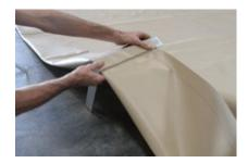
Slide the aluminum angles into pockets located on the walls of the berm so that the top portion of the angle fits into the pocket, while the bottom sits underneath the berm.
