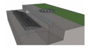
Step 2: Unfold and lay out Curb Inlet Filter with foam inserts facing you and overflow windows oriented on top. Carefully thread support rods through top and bottom channel pockets (Fig 1).
